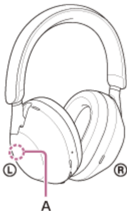
A: Location of the built-in antenna
