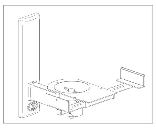
5 Place speaker on the platform, adjust clamps to hold speaker in place.
