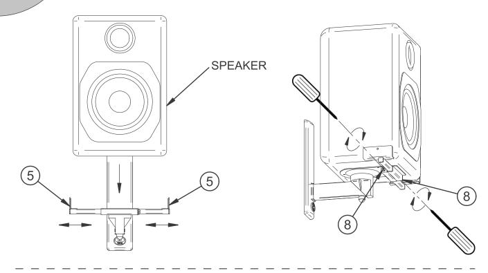
Where possible, avoid having front of speaker overhanging front of mount. If speaker must overhang, see table below for maximum overhang (distance A): **Note:** Maximum speaker dimensions *Height*.450mm / *Width*.280mm / *Depth*.350mm
