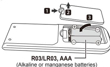
– Insert the batteries to the terminal so that it (+ and -) matches those in the remote control.
